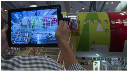
Figure 9d: AR structural damage location.
